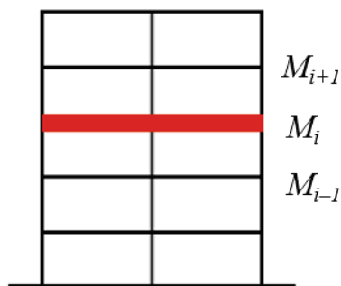
Figure 6-1 Mass irregularity per ASCE/SEI 7-16.
