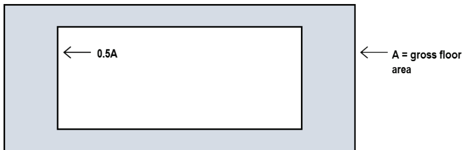
Figure 7-4 Diaphragm discontinuity comprising 50% of the gross floor area drawn to scale.
